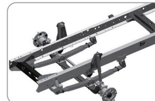
Front Parabolic Suspension and Rear Semi-elliptical Suspension
